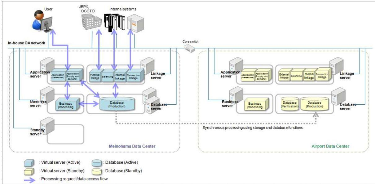
Fig. 1: Configuration of the Supply and Demand Adjustment Support System
